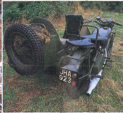
Sidecar mounted spare fits all three wheels. Quick change requires removal of three sleeve nuts and wheel spindle.
